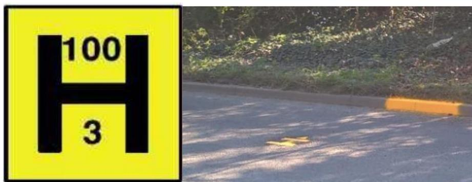
As well as marker plates, all hydrants are also shown on the digital maps available in fire engines, so that the nearest one can be found whilst firefighters are on their way to an incident. This also means that even if marker plates are missing or broken, the fire service will still be able to find them, and once reported they will be repaired in due course.
